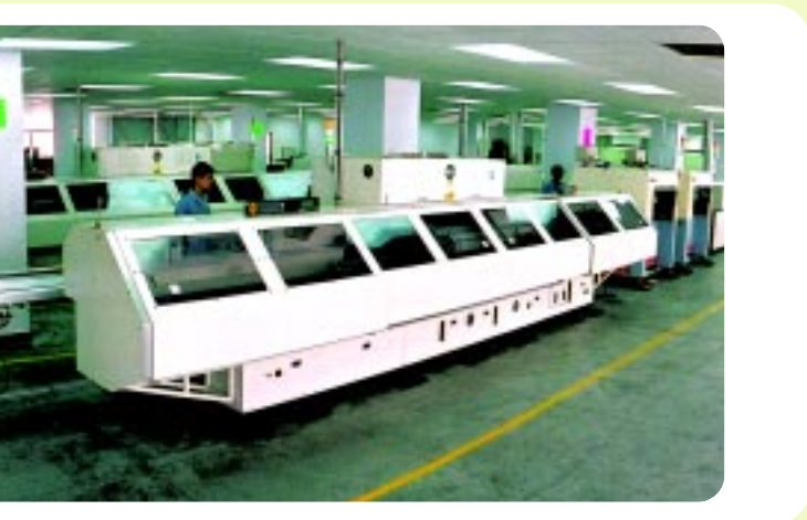
Advanced “Panaset MVIIF” SMT versatile placement machine.
