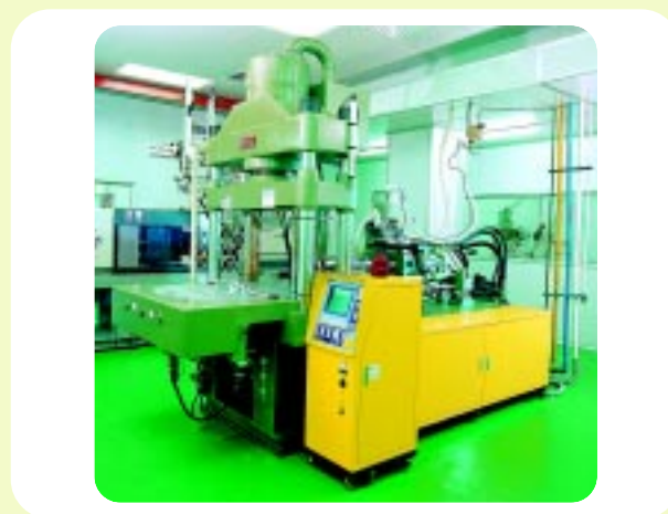
Dust free injection plant.
